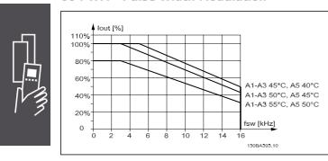
Derating of  $I_{\text{out}}$  for different  $T_{\text{AMB, MAX}}$  for enclosure A, using 60 PWM
