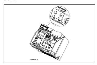
Connection to 24 V back-up supply on frame sizes A5, B1, B2, C1 and C2.
