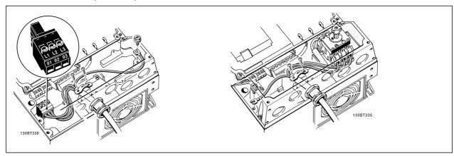
When disconnector is used (A5 enclosure) the PE must be mounted on the left side of the drive.
