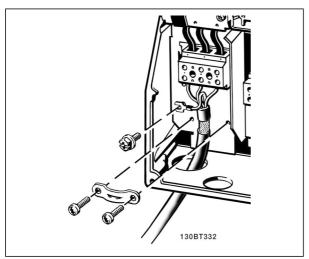
Mains connection C1 and C2 (IP 21/ NEMA Type 1 and IP 55/66/ NEMA Type 12) enclosures
