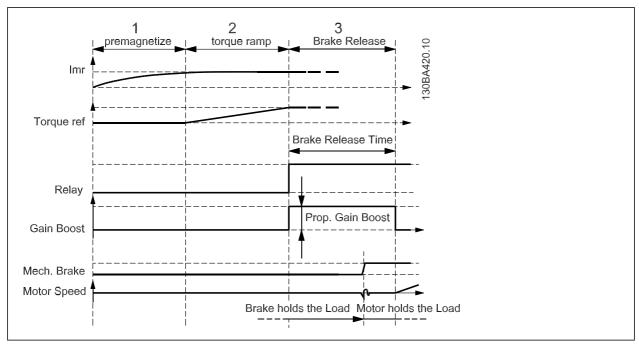
Brake release sequence for hoist mechanical brake control
