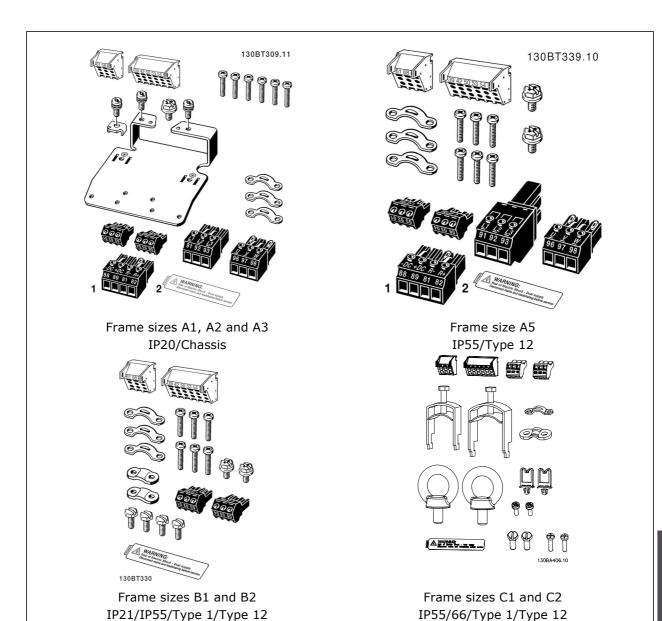
1+2 only available in units with brake chopper. Only one relay connector is included for FC 101/301 units. For DC link connection (Load sharing) the connector 1 can be ordered separately (Code no 130B1064)
