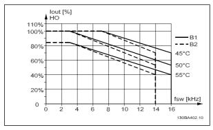
Derating of  $I_{\text{out}}$  for different  $T_{\text{AMB}}$ , MAX for enclosure B, using 60 PWM in High torque mode (160% over torque)
