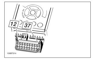
Bridge jumper between terminal 37 and 24 VDC
