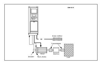
Basic Set-up for FC 302 Closed Loop Speed Control
