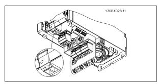
Connection to 24 V back-up supply on frame sizes A2 and A3.
