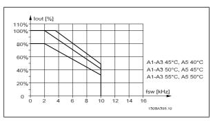
Derating of  $I_{\text{out}}$  for different  $T_{\text{AMB, MAX}}$  for enclosure A, using SFAVM
