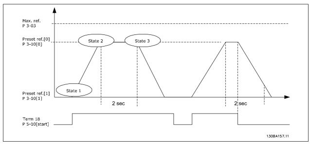
Set the ramping times in par. 3-41 and 3-42 to the wanted times
