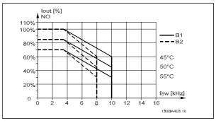
Derating of  $I_{\text{out}}$  for different  $T_{\text{AMB}}$ ,  $_{\text{MAX}}$  for enclosure B, using SFAVM in Normal torque mode (110% over torque)
