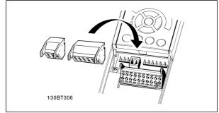
Assembling of IP55 / NEMA Type 12 (A5 housing) with mains disconnector
