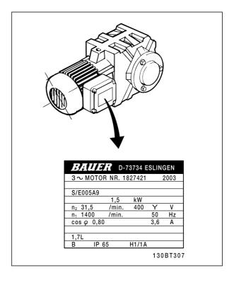
Step 2. Enter the motor name plate data in this parameter list.
