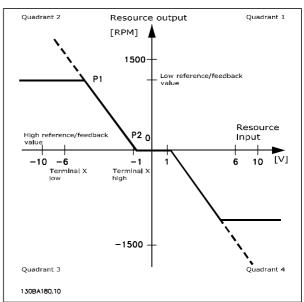
Thus a reference endpoint of P1 = (0 V, 0 RPM) will not result in any dead band, but a reference endpoint of e.g. P1 = (1V, 0 RPM) will result in a -1V to +1V dead band in this case provided that the end point P2 is placed in either Quadrant 1 or Quadrant 4.
