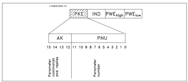
Bits no. 12-15 transfer parameter commands from master to slave and return processed slave responses to the master.
