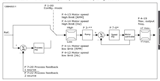
In the shown configuration, par. 1-01 *Motor Control Principle* is set to "Flux sensorless [2]" and par. 1-00 is set to "Speed open loop [0]". The resulting reference from the reference handling system is fed through the ramp and speed limitations as determined by the parameter settings indicated.
