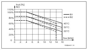
Derating of  $I_{\text{out}}$  for different  $T_{\text{AMB}}$ ,  $_{\text{MAX}}$  for enclosure B, using 60 PWM in Normal torque mode (110% over torque)
