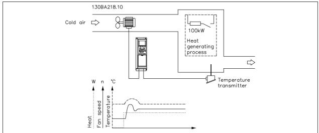
In a ventilation system, the temperature is to be settable from - 5 - 35°C with a potentiometer of 0-10 Volt. The set temperature must be kept constant, for which purpose the Process Control is to be used.
