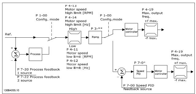
In the configuration shown in the illustration above, par. 1-01 *Motor Control Principle* is set to "VVC<sup>plus</sup> [1]" and par. 1-00 is set to "Speed open loop [0]". The resulting reference from the reference handling system is received and fed through the ramp limitation and speed limitation before being sent to the motor control. The output of the motor control is then limited by the maximum frequency limit.
