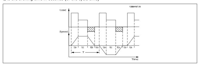
Danfoss offers brake resistors with duty cycle of 5%, 10% and 40%. If a 10% duty cycle is applied, the brake resistors are able to absorb brake power for 10% of the cycle time. The remaining 90% of the cycle time will be used on dissipating excess heat.
