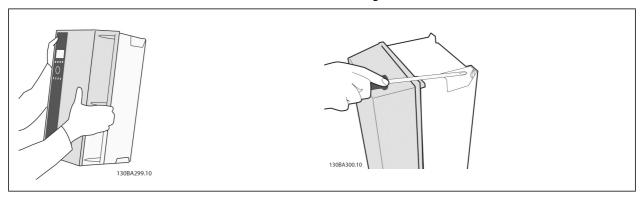
Mounting frame sizes A5, B1, B2, C1 and C2 on a non-solid back wall, the drive must be provided
