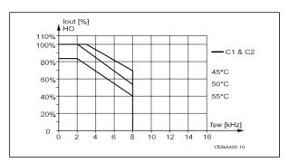
Derating of  $I_{\text{out}}$  for different  $T_{\text{AMB, MAX}}$  for enclosure C, using SFAVM in High torque mode (160% over torque)
