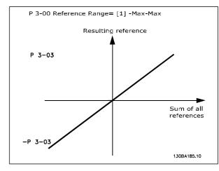
The value of par. 3-02 *Minimum Reference* can not be set to less than 0, unless the par. 1-00 *Configuration Mode* is set to [3] Process. In that case the following relations between the resulting reference (after clamping) and the sum of all references is as shown to the right.
