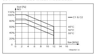
Derating of  $I_{\text{out}}$  for different Tamb, Max for enclosure C, using 60 PWM in Normal torque mode (110% over torque)
