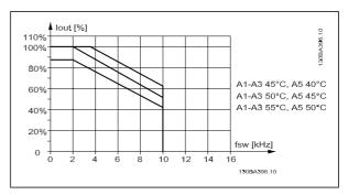
Derating of  $I_{\text{out}}$  for different Tamb,  $_{\text{MAX}}$  for enclosure A, using SFAVM and maximum 10 m motor cable
