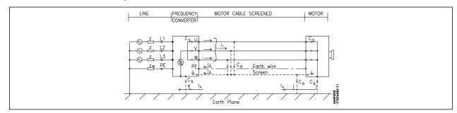
If the screen is to be placed on a mounting plate for the frequency converter, the mounting plate must be made of metal, because the screen currents have to be conveyed back to the unit. Moreover, ensure good electrical contact from the mounting plate through the mounting screws to the frequency converter chassis.
