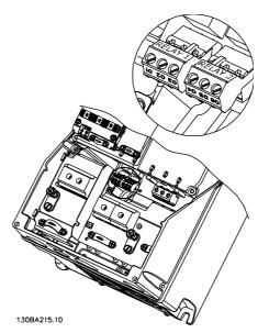
Terminals for relay connection (Frame sizes A5, B1, B2, C1 and C2).
