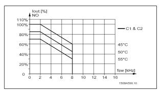
Derating of  $I_{\text{Out}}$  for different Tamb, max for enclosure C, using SFAVM in Normal torque mode (110% over torque)
