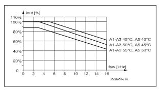
Derating of  $I_{\text{Out}}$  for different T\_AMB, MAX for enclosure A, using 60 PWM and maximum 10 m motor cable
