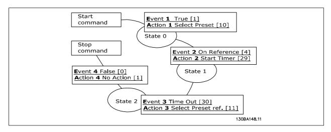
Set the Smart Logic Control in par. 13-00 to ON.
