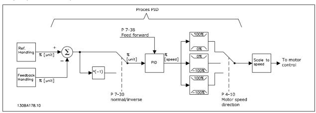
**Process PID Control diagram**
