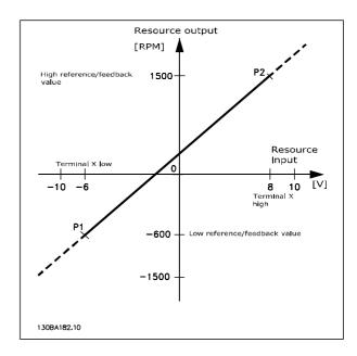
The endpoints P1 and P2 are defined by the following parameters depending on which analog or pulse input is used
